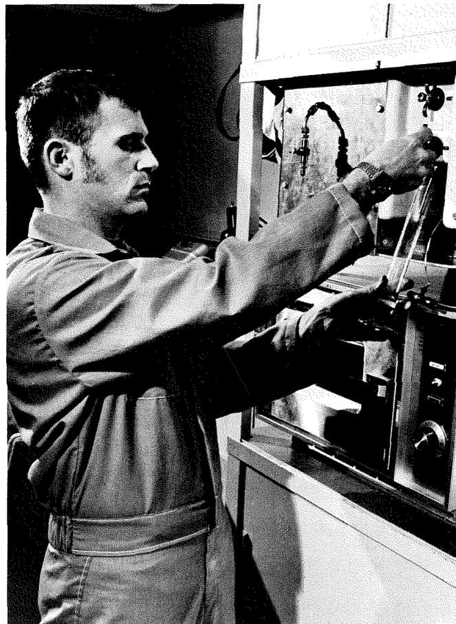
*To keep track of water consumption, John Hall measures the amount he is withdrawing from the potable water dispenser. Water, recovered from the crew's urine, perspiration, and wash water, was purified for reuse.*
