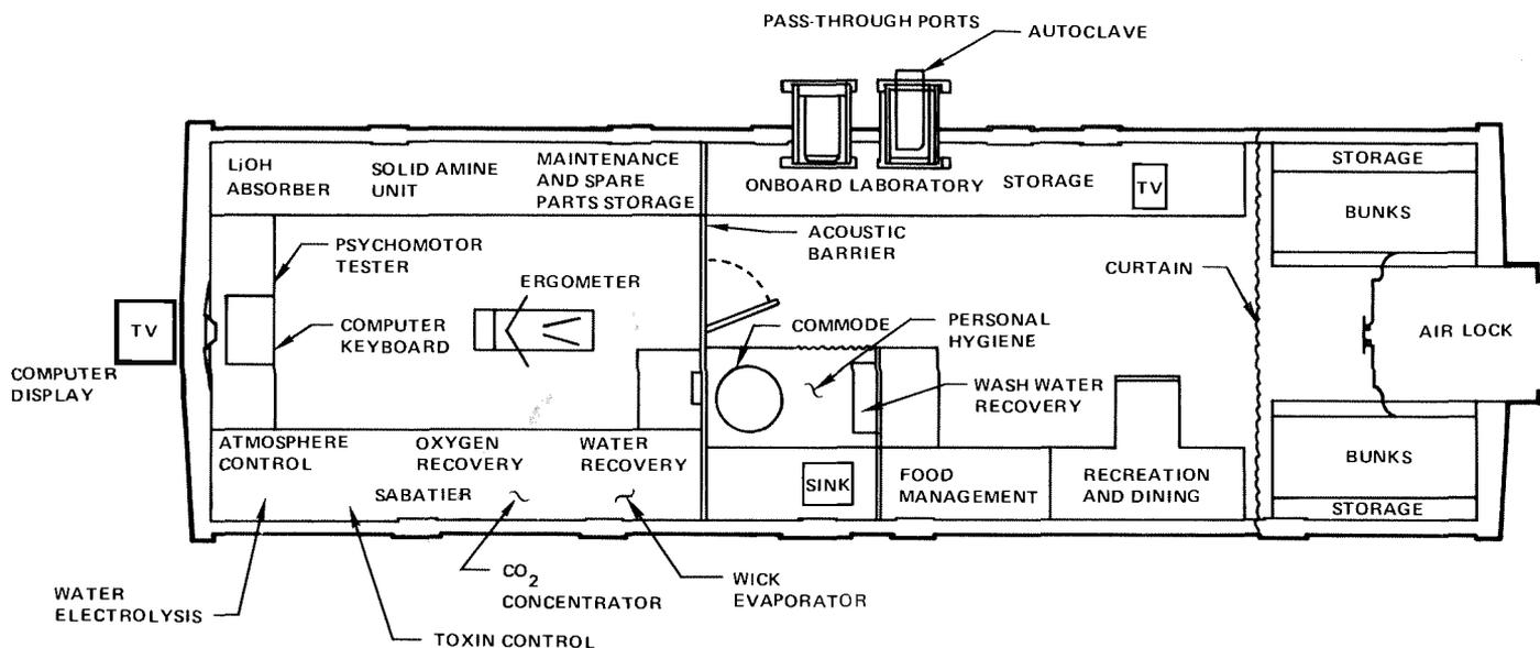
The floor plan of the 40-foot-long "home" for the four crewmen is a testament to careful planning and ingenuity in stowing a large amount of equipment into a compact area.
