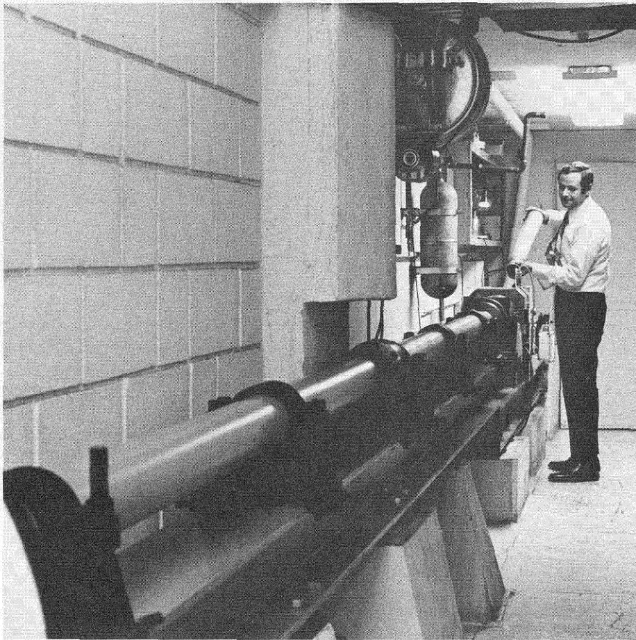
Thomas Ahrens, associate professor of geophysics, loads his converted Navy cannon. At the end of its 24-foot-long barrel is a 120-cubic-foot vacuum tank in which the target mineral is suspended.
