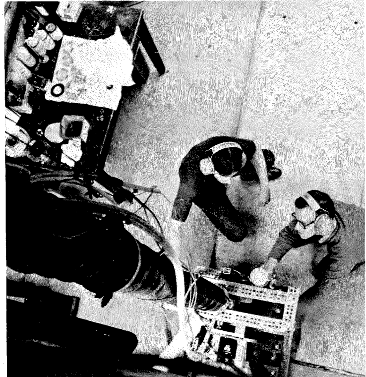
The ear-splitting noise of a motorcycle engine attached to an open-ended acoustical pipe demands distance or discretion. Brad Sturtevant and his co-workers wisely choose to wear heavy ear pads.
