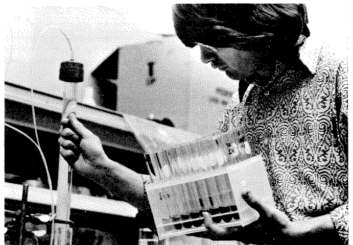
Fensom processes the liquid several times through a series of filtration columns to separate the proteins on the basis of electric properties and molecular weight. The resulting liquid, now dark blue, is pure copper protein—plastocyanin.
