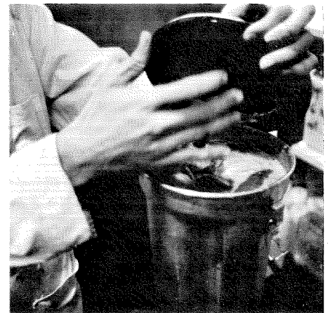
Each bag of leaves was reduced to a green liquid mush in a blender. The fibrous residue was filtered out by pouring the mixture through a porous plastic material.
