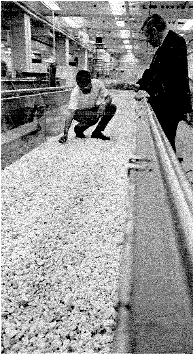
Josephat Okoye, one of the first students to earn a PhD in environmental engineering science, and Norman Brooks, professor of environmental science and civil engineering—and coordinator of the EES program—prepare a flume for use in studies of pollution patterns in stream beds.
