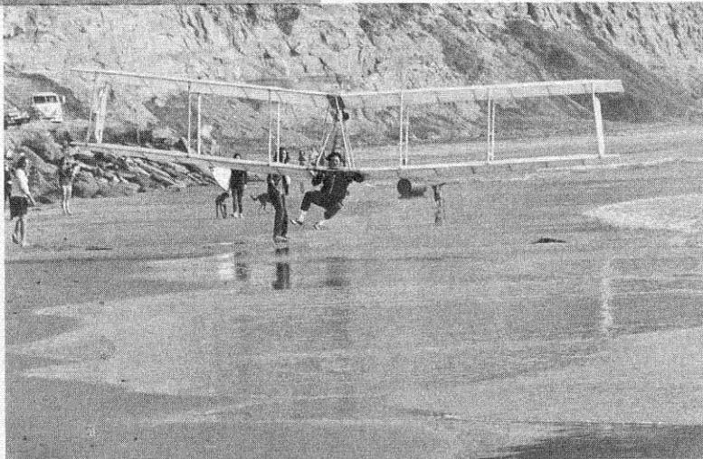
At the end of the flight, Taras brings *Icarus* in for a gentle landing. He braces his feet on the aluminum tubing and swings backward and forward in the seat sling to control the glider. A final backward motion brings the front of the glider up enough to slow his speed for a comfortable landing. Then, dropping his feet, he calmly walks to a stop.
