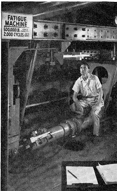
Ralph Oliva, research engineer, examines Super Constellation skin for signs of fatigue failure.
