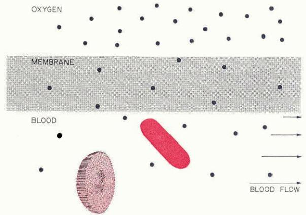
*Schematic diagram of the oxygen-membrane-blood interfaces in the artificial lung. The film of slowly moving blood at the membrane surface inhibits oxygen absorption. Shown also are two red cells (viewed from different angles) with the one nearer the membrane more highly oxygenated.*
