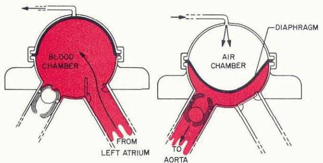
*A schematic diagram of an artificial heart, designed to carry part of the pumping load for a period of days after a patient has undergone heart surgery. The diagram on the left shows the heart as blood is drawn in, and the one on the right as it is pumped into the aorta.*
