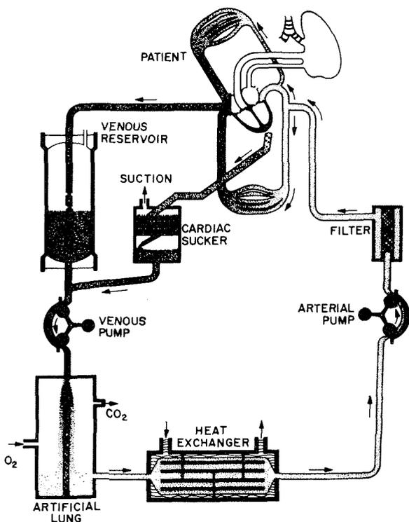
External circulatory system of a type used in heart surgery (from Heart-Lung Bypass by Galletti and Brecher, Grune and Stratton, New York, 1962).
