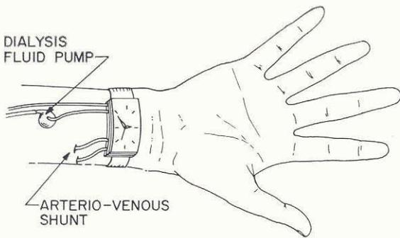
*Artificial kidney of the future, as envisioned by Dr. L. W. Bluemle, Jr., of the University of Pennsylvania. The device would work continuously as part of the arterio-venous shunt using dialyzing fluid from a reservoir located on the patient's body.*
