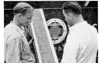
1500 feet of formation is accurately charted by Lane-Wells Electrolog.
