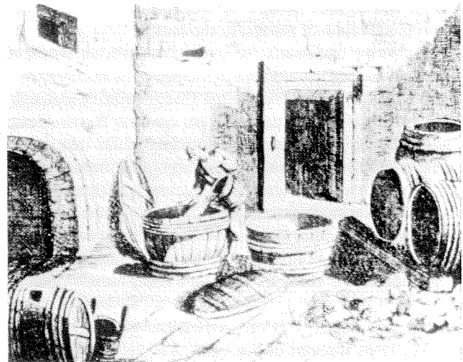
Early vinegar manufacturing processes used shallow vats; the chemical reactions involved in vinegar production required large open surfaces for oxygen supply and release of heat.
