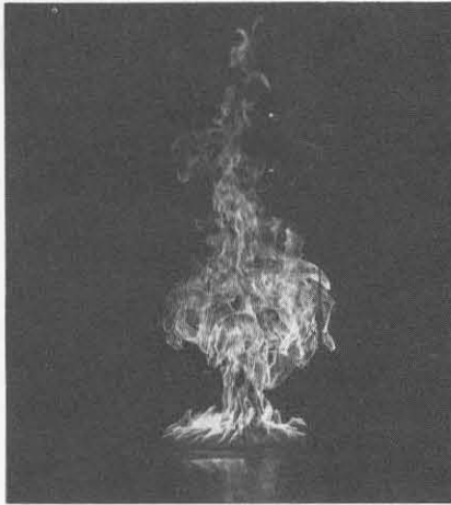
When a vortex-like puff that has risen to the top of the flame burns off (left), the top of the flame drops to the next puff.
