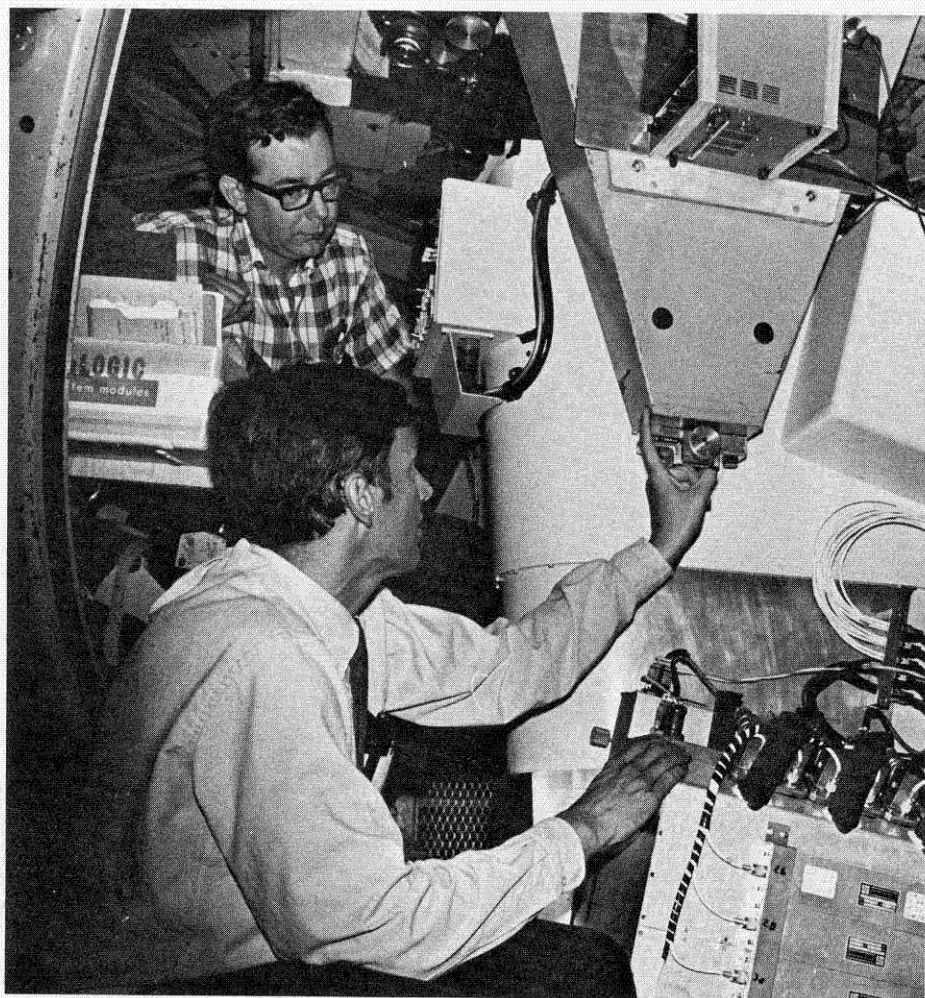
The 32-channel spectrometer on the 200-inch Hale telescope at Palomar is one of several new systems for increasing the observational efficiency of the instrument. Edwin Dennison, director of the Astro-Electronics Laboratory, and J. Beverley Oke, professor of astronomy and associate director of the Hale Observatories, make a few adjustments in preparation for the night's observations.
