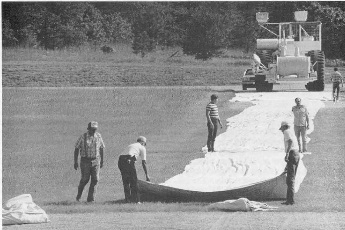
Technicians lay out a clean ground cloth from Tiny Tim to the edge of the launch pad for the empty balloon to lie on. Even a twig could pierce the balloon's delicate skin.
