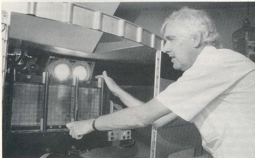
Ronald Scott adjusts the earthquake basket of the centrifuge. A model of, say, a dam, set into the basket, can be shaken like a model earthquake (compressed into .2 seconds), reflected in the mirror angled above the basket, and filmed by a high-speed movie camera that uses 100 feet of film in 3 to 4 seconds.
