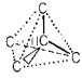
Figure 1: Carbon in diamond is bonded to four atoms arranged in a tetrahedron.
