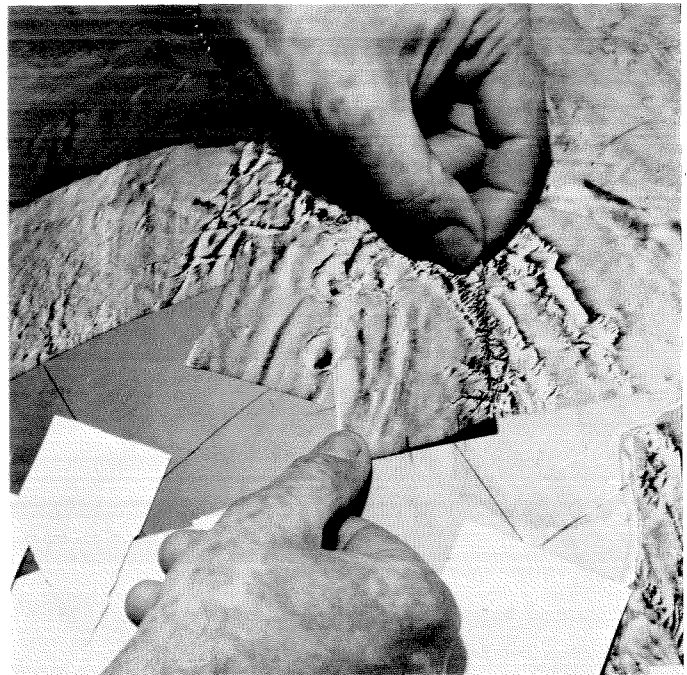
Gluing down a section is perhaps the most delicate step in the whole process. To do exact matching, a scalpel-like blade is used to trim overlapping sections along feature lines, so that each blends imperceptibly with the others around it.
