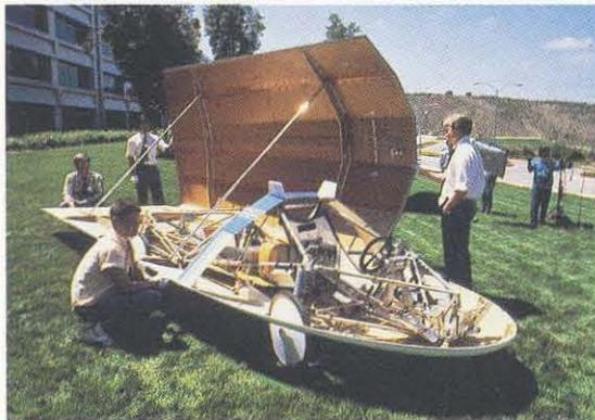
Left: the lightness of the chassis and emptiness of the interior are apparent when the canopy is removed and the solar-array panel tilted up.
