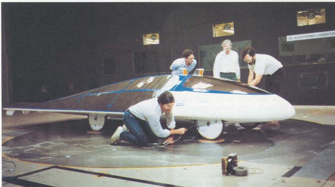
An AeroVironment crew checks out the Sunraycer prototype during tests in the GM wind tunnel. There were no surprises, but the tests quantified the effects of many small cleanups, making it possible to decide which ones justified being incorporated into the race vehicle.
