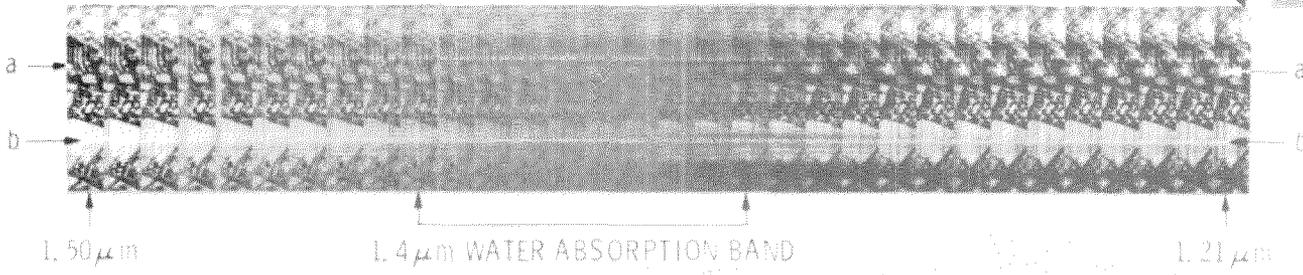
**Air photo and spectral image showing (a) a school courtyard and (b) an open field in Van Nuys, California. The black rectangle outlines the area covered at 32 wavelengths between 1.5 and 1.21 microns. The well-watered courtyard shows a different reflectance pattern than the drier field. The gray blur at 1.4 microns is due to atmospheric water vapor.**
