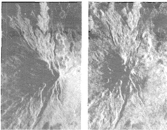
**This 3-D view of Mt. Shasta was created from a pair of Shuttle Imaging Radar images taken at 29° from vertical (right) and 60° from vertical (far right).**
