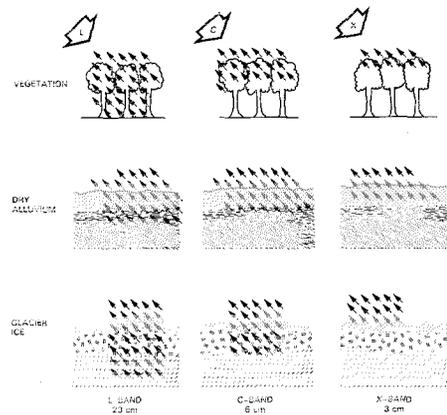
**Microwave radars penetrate to different depths, depending on the wavelength.**
