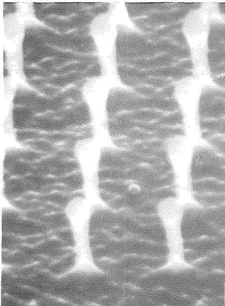
**Above: An orchard of quantum dots. The bulbous dots, 0.05 microns in diameter, sit on gallium arsenide stalks spaced 0.38 microns apart. Right: The piezoelectric walker. Each leg of the triangle is 1.5 inches long. The rod on the right apex carries the needle; the chip bearing the quantum dots is the tiny black square in the mounting to the walker's right. The optical fiber goes off to the right.**
