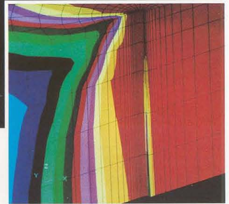
Above: A supercomputer model of the stresses around the crack, which is moving from left to right across the face of the model. Blue is the lowest stress, red the highest. The inset shows that bonds breaking at the crack tip relieve stress in the immediate area. Below: A typical interference pattern. The crack is moving up the middle of the photo.
