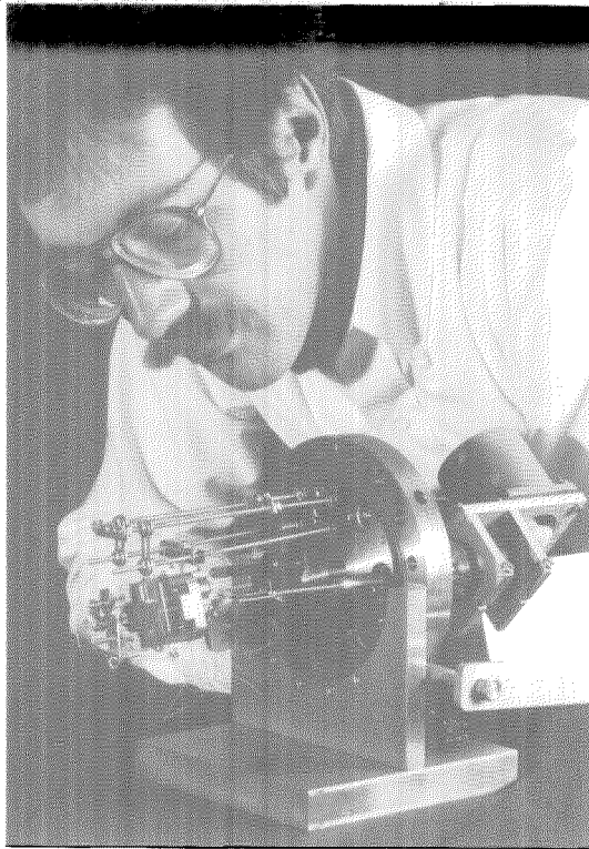
The ballistic electron emission microscope (BEEM), shown here with Bill Kaiser, provides a new view below the surface. Below: The surface of a gold/gallium arsenide structure is revealed by STM (top) and the interface of the two materials by BEEM (bottom).
