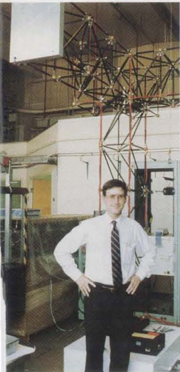
Fanson and the Lab's latest active structure. The 11-inch by 16-inch trusswork weighs 50 pounds. The test mass at the arm's end weighs 52 pounds. The whole structure is built on a 3500-pound base to eliminate outside vibrations.
