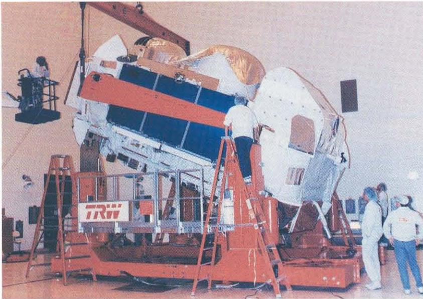
**Workers in the Payload Hazardous Servicing Facility at Kennedy Space Center carefully position the massive Compton Gamma-Ray Observatory on a test stand. Deployed April 7, 1991 from the shuttle *Atlantis*, the 35,000-pound observatory carries four instruments to study celestial gamma-ray sources.**
