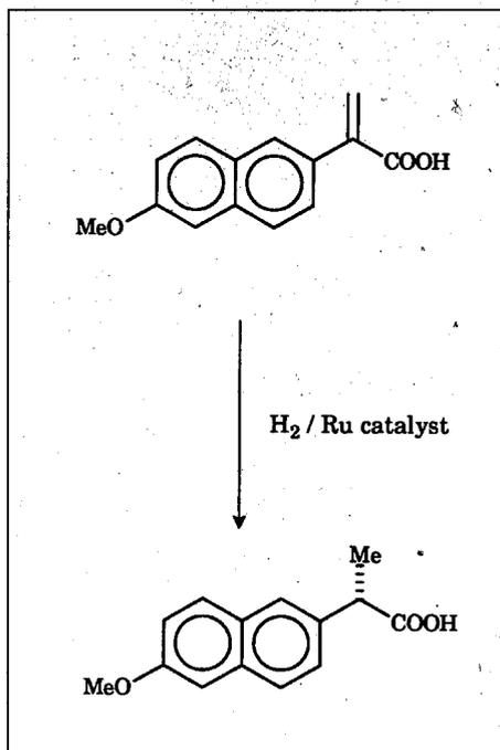
**Above: The final step in synthesizing naproxen. The planar precursor molecule (top) is achiral. The chiral naproxen molecule (bottom) has its methyl group (Me) behind the plane of the page in the "good" form; in the toxic form the methyl group sticks out in front of the page.**
