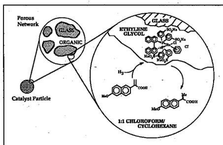
medium does, a little brisk stirring coats the beads with a very thin layer of the catalyst-containing solvent. Since the catalyst is fully dissolved in a liquid, the organic shrubbery is free to take its preferred shape, and as the solvent layer is very thin, the catalyst is close enough to the reaction medium to slurp up the starting ingredients, run the reaction, and spit the finished products back into the reaction medium.
