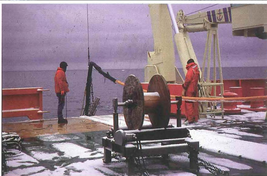
Members of the crew deploy the seismic streamer off the Nathaniel B. Palmer's rear deck, a precarious place to be in rougher weather than this. The ship also towed a magnetometer behind it, and mounted on the ship itself are a gravity meter and an array of instruments to map a three-dimensional swath of the seafloor beneath the ship (below).
