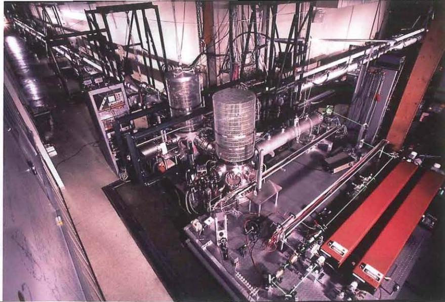
The prototype interferometer, a hundredth the size of the monster on page 8, was begun in the early '80s on the Caltech campus. The green laser beam generated from the optical setup at lower right enters the system through the horizontal pipe (center), and from the beam splitter in the mesh cage is bounced down the 40-meter arms.
