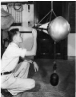
In his early years at Caltech, Leighton designed this cosmic ray detector to be flown on a balloon.
