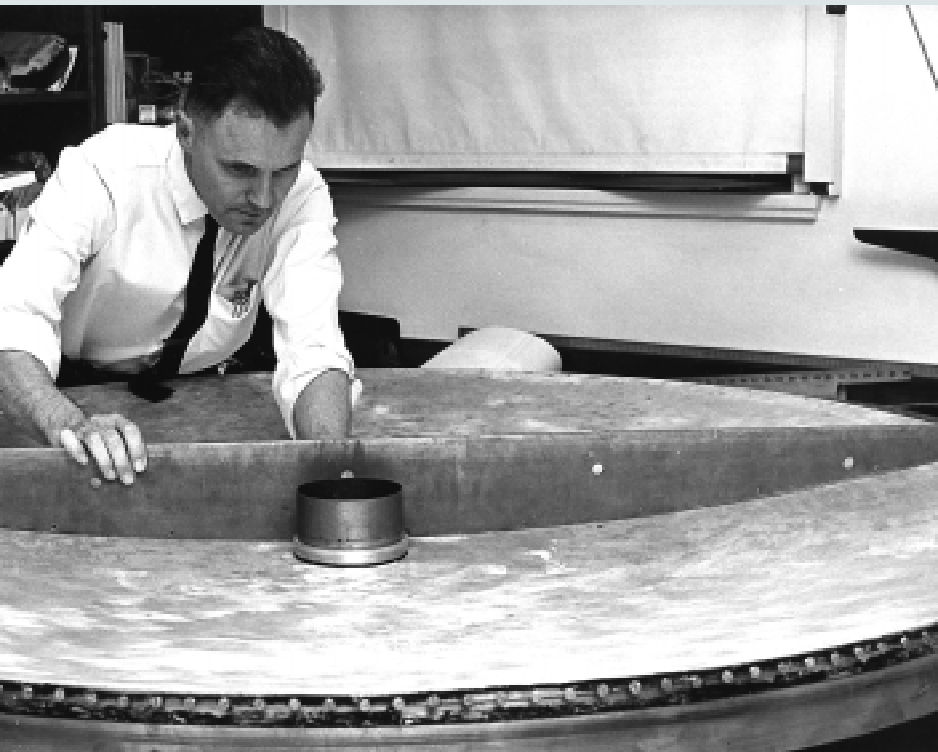
In the early '60s, Leighton sculpts the surface of the first infrared telescope, which is now in the Smithsonian Museum. At 62 inches, it was once the second largest telescope on Mount Wilson.
