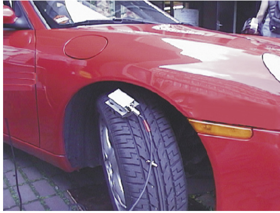
A prototype of the NMR-MOUSE testing a tire.
