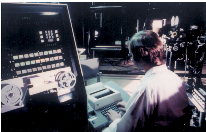
Feeney as an undergrad with one of his and Holland’s computer-controlled camera stands. This one was used for animating logos for commercials. The camera (visible at far right over Feeney’s shoulder) points at an illuminated glass table, on which artwork and colored gels were placed to be photographed.
