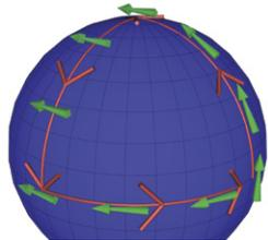
**The red line follows a round trip made on a curved surface by a traveler holding a gyroscope. On returning to the starting point, the spin axis of the gyroscope (green arrow) would have turned 90 degrees from its original heading. Similarly, a satellite orbiting Earth travels through the curved space-time around it and, with each orbit, the orientation of the satellite changes slightly.**
