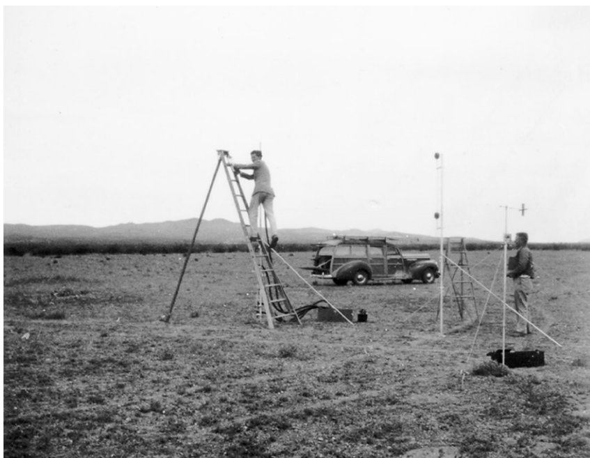
Otvos (on ladder) and Johnston set up the micro-meteorological gear near Rosamond Dry Lake in the Mojave Desert some time in 1943. The thermocouple mast and its suction system are visible behind Otvos' ladder. The center mast has two anemometers on it, and the mast in front of Johnston carries a British gustiness meter. Note the Buick in the background.
