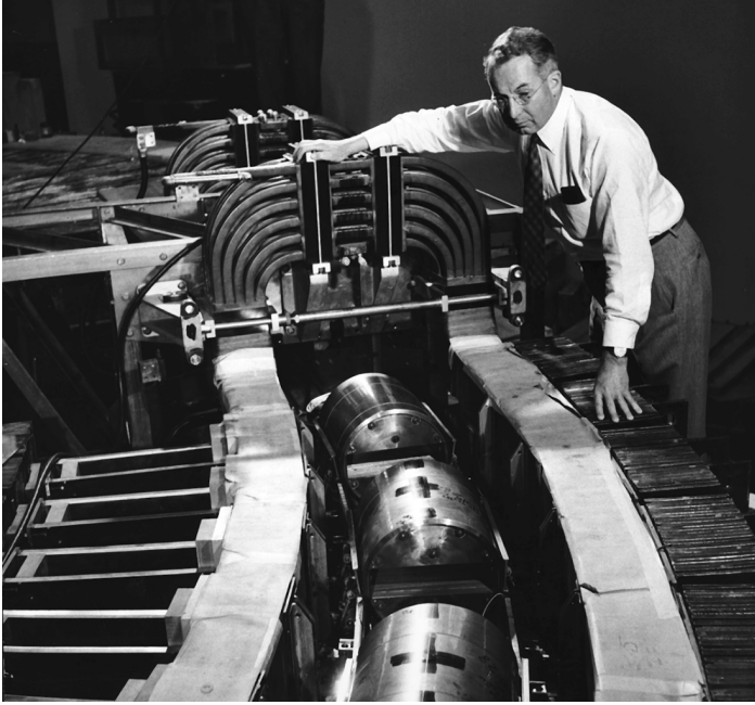
Bacher stands beside the magnet of the synchrotron in 1955. At that time the electron accelerator had a peak energy of about 300 MeV; Phase 2, which began operation in 1957 had a peak energy of just over a billion volts.
