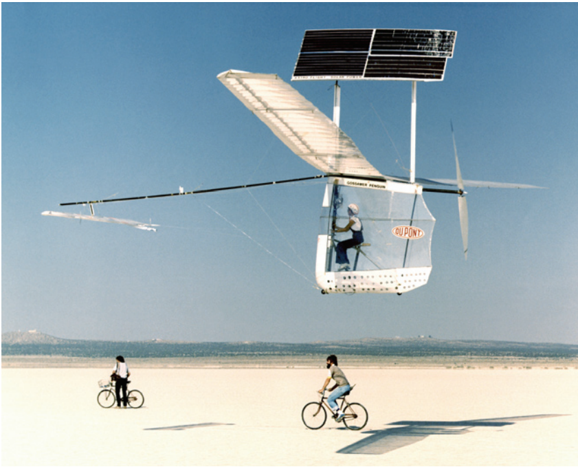
AeroVironment's Gossamer Penguin, a three-quarter-scale, solar-powered version of the Gossamer Albatross, takes wing over Rogers Dry Lake bed in the summer of 1980. The Penguin was the prototype for AeroVironment's Solar Challenger and Helios—the latter holding the world altitude record for any steady-flying (as opposed to ballistically climbing) airplane. It soared to 96,863 feet, two miles higher than the SR-71 "Blackbird" it beat.
