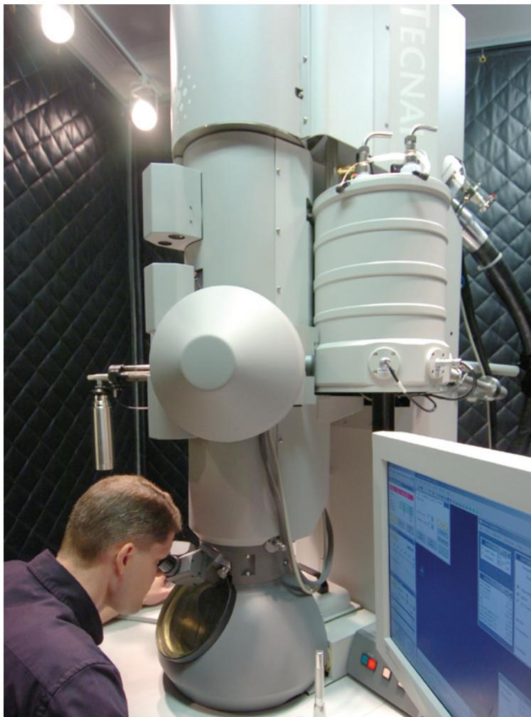
Jensen and the lab's 300-kilo-electron-volt (keV) transmission electron microscope, a liquid-helium-cooled Polara G2. The eyepiece is used for rough positioning of the sample in the vacuum chamber; the actual images will appear on the monitor to his right. The quilted black panels in the background completely surround the apparatus and are part of the airflow-management system.
