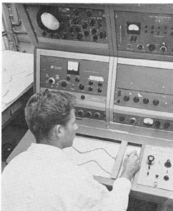
Edward Glazer determines a nuclear magnetic spectrum. The sample is in an adjoining 12-inch electromagnet. The spectrum recorded at the console will later be compared with other spectra of the same material taken at different temperatures.
