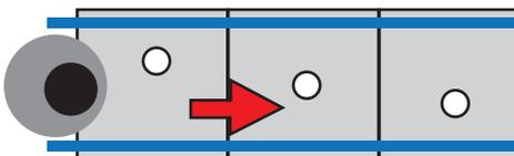
The diagonal arrangement of the holes allows the CCD to take a picture of different parts of the specimen at different times as it flows by. The diagonal arrangement keeps a one-to-one correspondence between each pixel and hole. Computer software puts the image slices together to create a complete picture.
