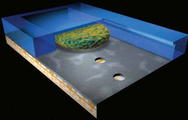
An up-close representation of the optofluidic microscope. The green specimen flows across the gray metal sheet. The detector underneath captures images of the specimen through the holes.
