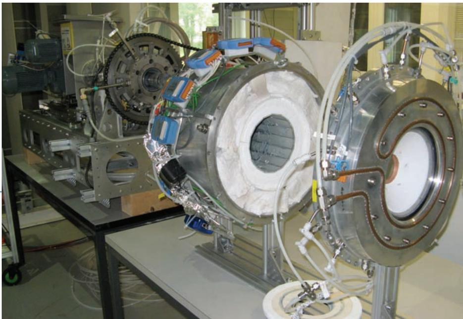
Steinfeld's 10-kilowatt zinc reactor operates at 2,000 kelvins. In the middle of the picture is the rotating reaction cavity, where the zinc oxide particles are held against the heavily insulated chamber wall by centrifugal force. The concentrated sunlight enters through the quartz window on the right, inside the copper C of cooling-water lines.
