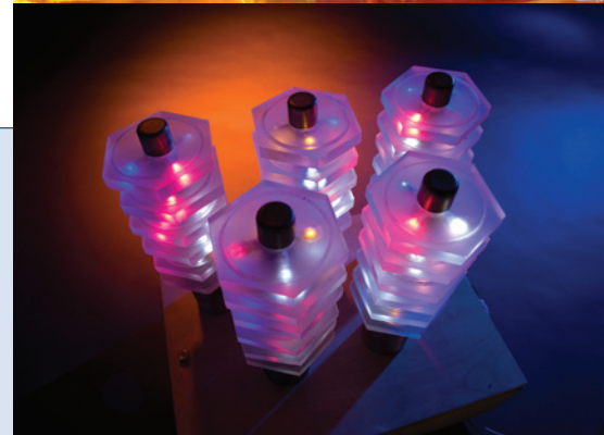
Top right: A top view of the five stacks that make up the CDMS experiment. Copper provides a first layer of protection against background particles.
