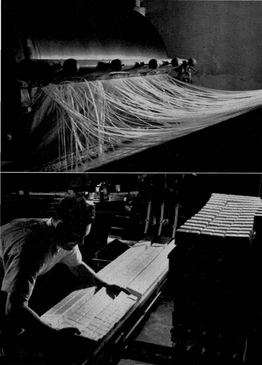
**FIG. 3.** Soap products are tailored for many specialized uses. Here paper-thin ribbons of soap are feeding off a huge roll into a drying oven on their way to becoming flakes. **FIG. 4.** Here three conveyor belts are feeding bars to a high-speed stamping machine. A watchful eye for quality is part of the stamp-feeder's job.
