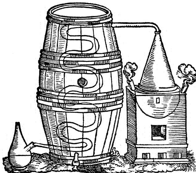
FIG. 3. Distillation apparatus with condenser tubes. Reproduced from Gildemeister and Hoffmann, Die Atherischen Ole , p. 226 (1910).
