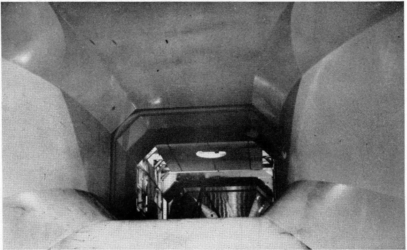
FIG. 21. View showing contraction entrance to working section.
