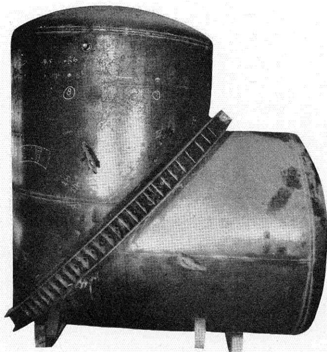
FIG. 7. Model of corner with elliptical ring.
