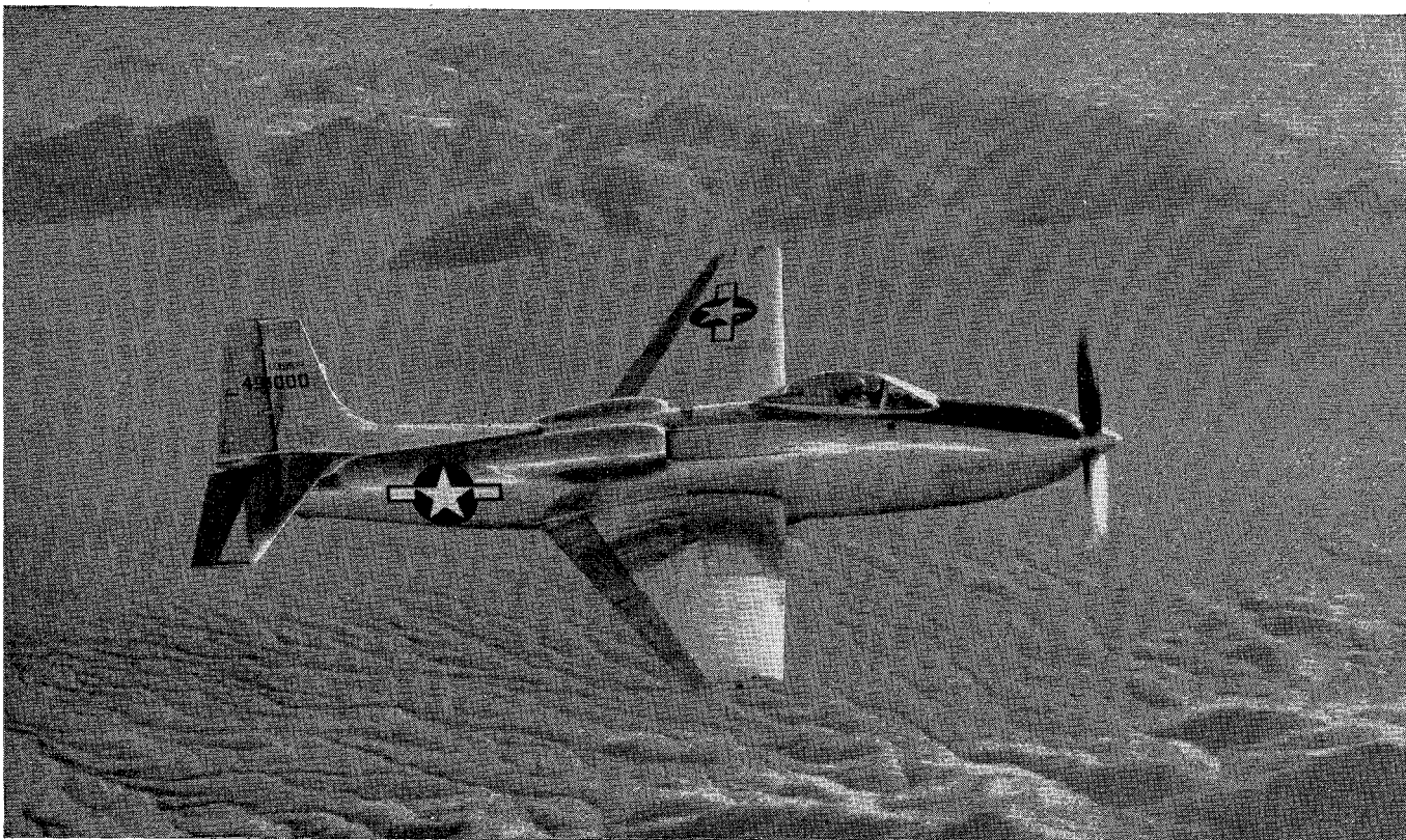
FIG. 1. The XP-81 shown above is the Army's latest fighter. Designed to escort B-29's on long range missions, it utilizes a gas turbine driving a propeller for cruising, plus a pure jet gas turbine for take-off and combat.
