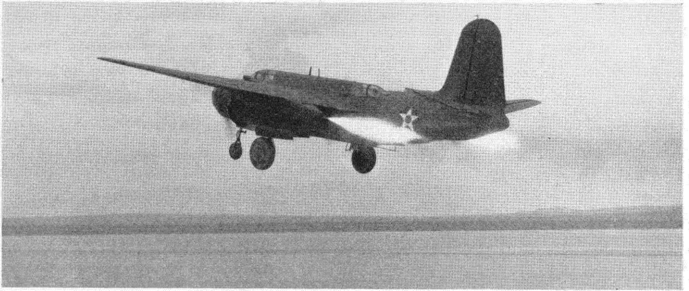
FIG. 5. A bi-motor Douglas bomber, the A-20A, takes off assisted by two 1,000 pound thrust, 25 second duration liquid motors.
