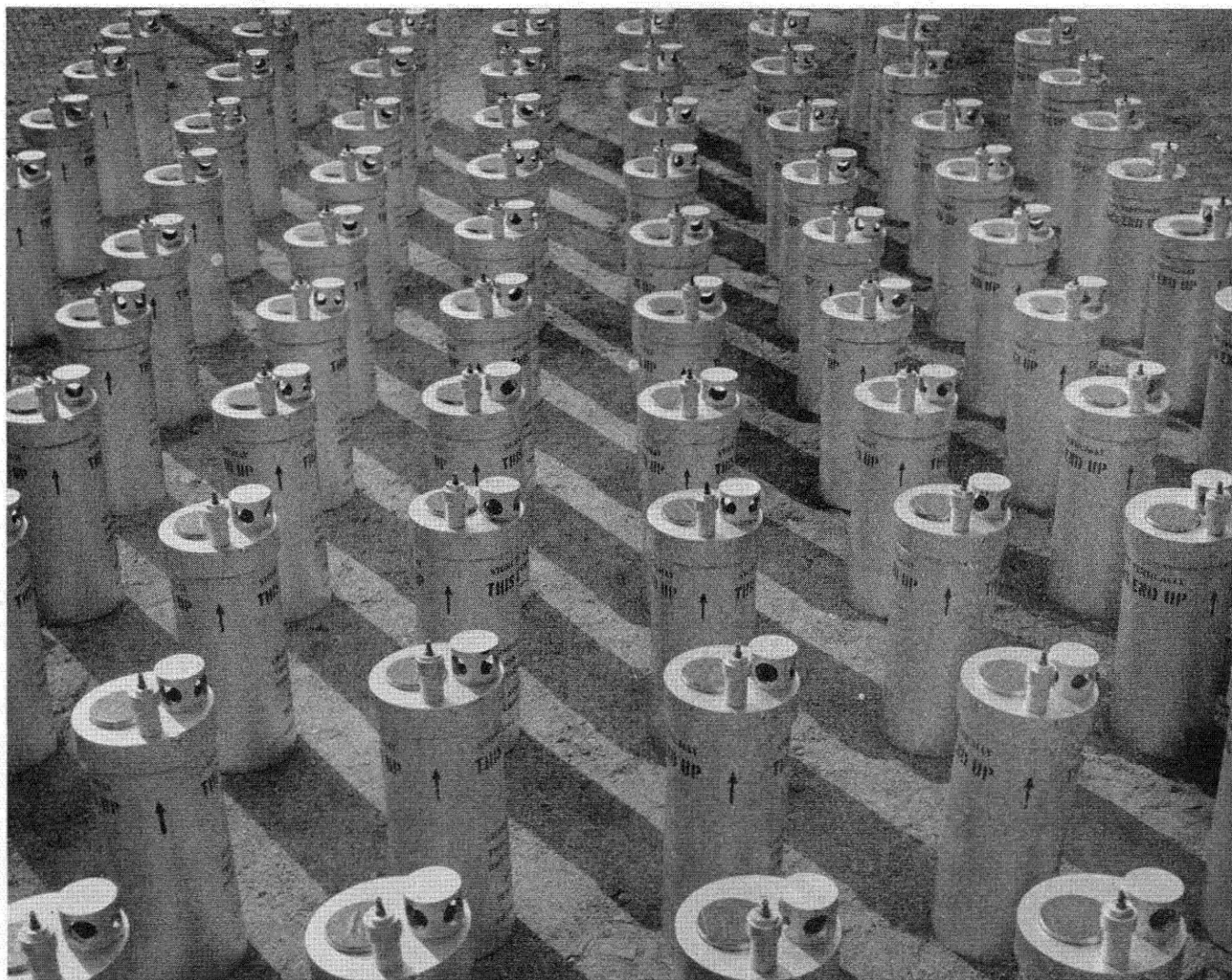
FIG. 4. Motors with 200 pound thrust, 8 second duration, ready for delivery to the U. S. Navy.
