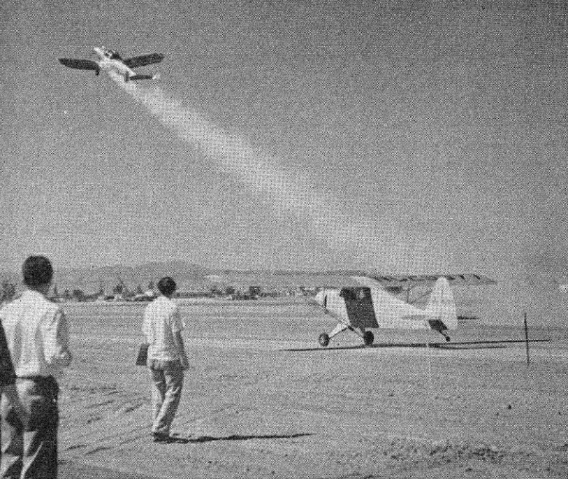
FIG. 3. Ercoupe take-off assisted, versus Porterfield take-off unassisted.
