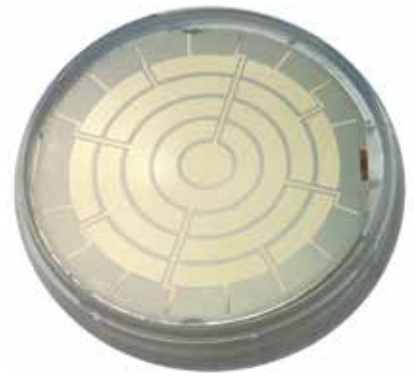
This early prototype of a deformable mirror was used by researchers to test the concept of AAReST.
