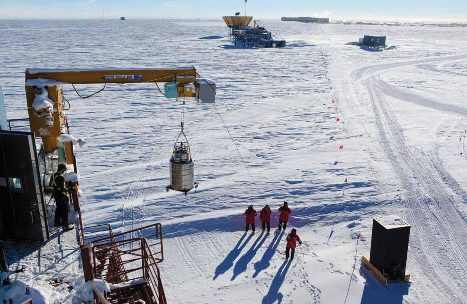
*BICEP2 team members lift a liquid helium cryostat to the second floor of the Dark Sector Laboratory to chill the telescope to a temperature near absolute zero.*
