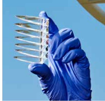
In the spectrum-splitting optical prototype for high efficiency solar cells pictured above, incident sunlight is divided into different frequency bands by the stack of filters. Each band of light is concentrated by a triangular silicone concentrator before conversion in the solar cell best tuned to that band.
