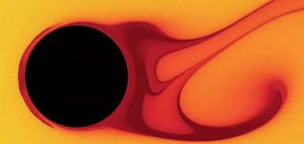
**THE VORTEX STREET** The image above is known as a Kármán vortex street—a repeating pattern of swirls (vortices) caused by an instability in the flow of a fluid as it passes over an object with a broad, flattened front called a bluff body. The phenomenon is named after Theodore von Kármán, the aerodynamics pioneer who was the founding director of what is now known as the Graduate Aerospace Laboratories at the California Institute of Technology (GALCIT).
