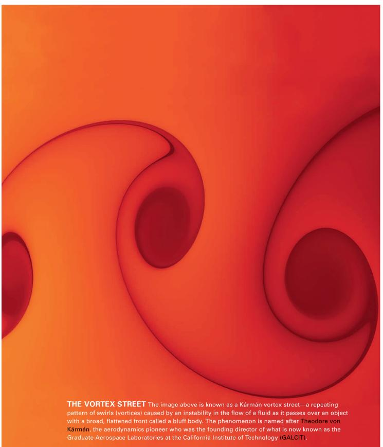
Unlike most such images—in which the swirls would have been visualized thanks to dye injected into a stream of fluid—this version was created by computer (and by mechanical engineer Tim Colonius), using numerical data from a simulation that tracked individual particles as they moved and tumbled past one another.
