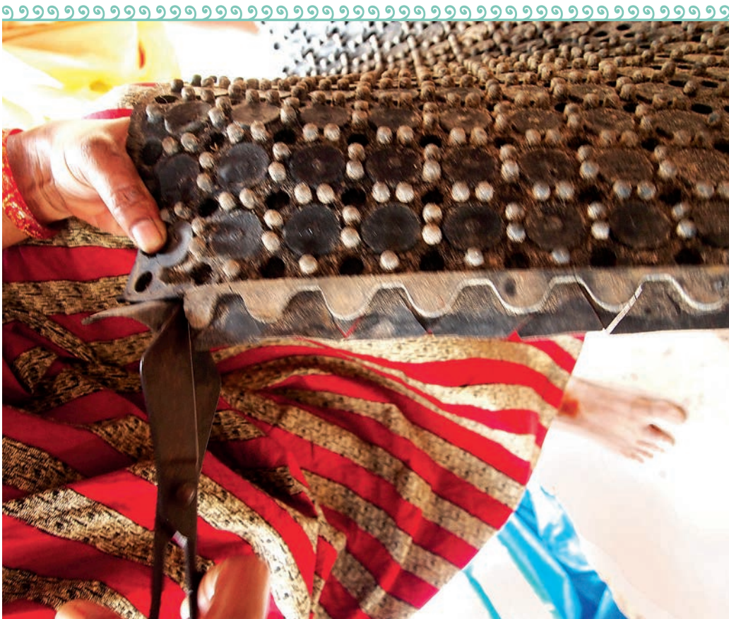
A woman at the Akhil Rubber Mat Works cuts excess rubber from a mat. Each of the approximately 150 holes in the mat must be chiseled out by hand, causing pain and strain for the workers.
